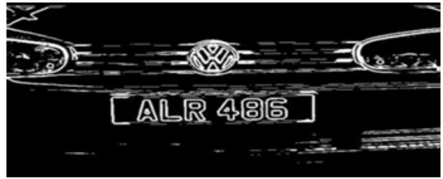
Fig. 9. Removing Horizontal Component & Detection of number
