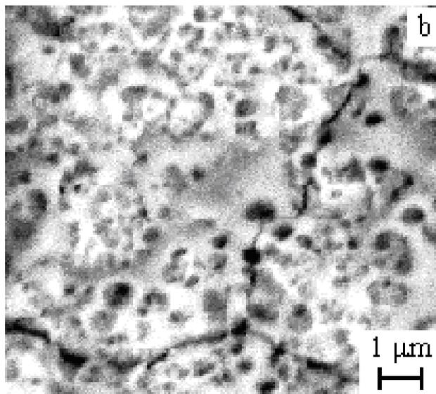
**Fig. 5. The images of the titanium cathode after the effect of the discharge in the electrolyte: a) sphere-like formations; b) pores structure of the surface**
