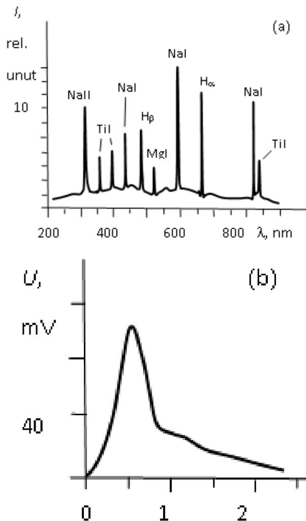
**Fig. 4. Radiation of the discharge in the electrolyte on the basis of sodium hydroxide:**
