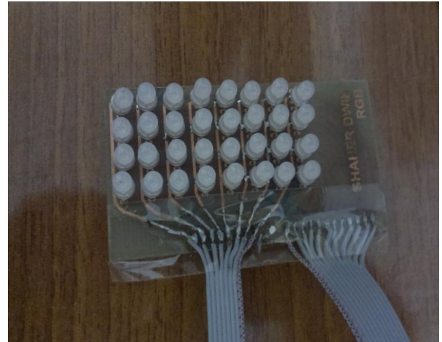
Fig.11: Fabricated RGB matrix display
