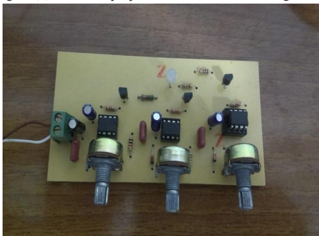
Fig.7: Fabricated driving circuit for single RGB LED
