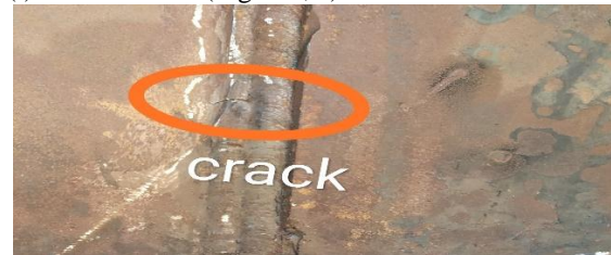
Fig. 13, a: linear cracks located on specimen surface.
