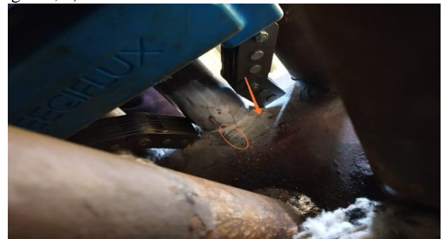
Fig. 13, b: rounded indication located on specimen
