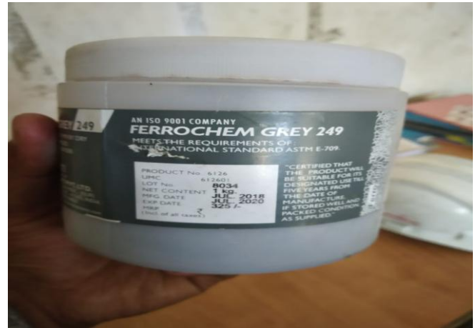
Fig. 9: Non-fluorescent dry method magnetic powder-Ferrochem Grey 249, ASTM E-709
