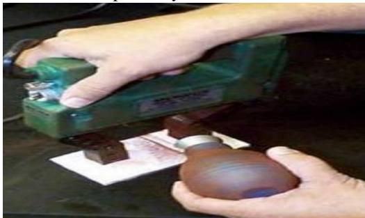
Fig. 11: Magnetic medium is applied on specimen with air blower
