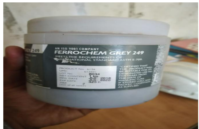
Fig. 9: Non-fluorescent dry method magnetic powder-Ferrochem Grey 249, ASTM E-709
