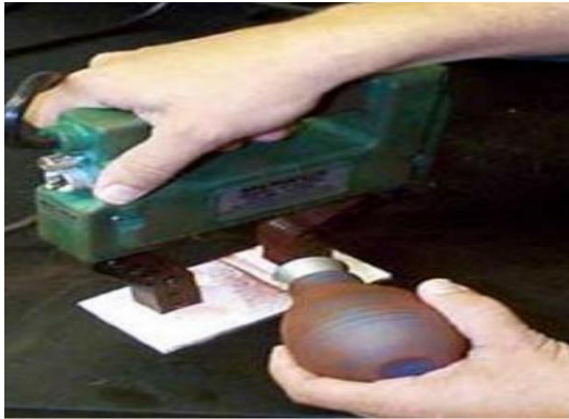
Fig. 11: Magnetic medium is applied on specimen with air blower
