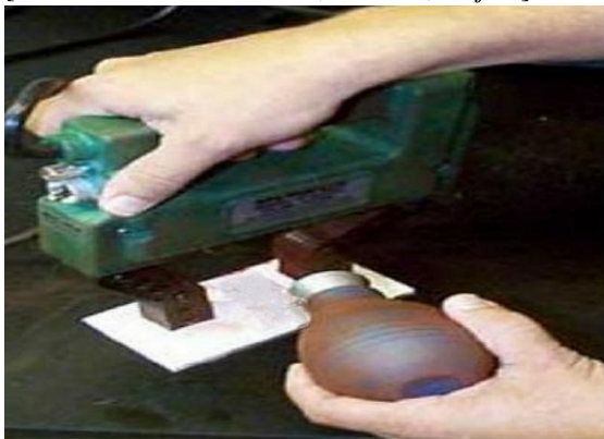
Fig. 12: Excess of medium removed from specimen with air blower.
