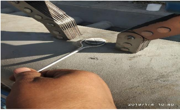
Fig. 7: pie gauge shows the magnetic strength
