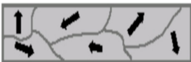
Fig. 2: Atoms of Unmagnetized material
