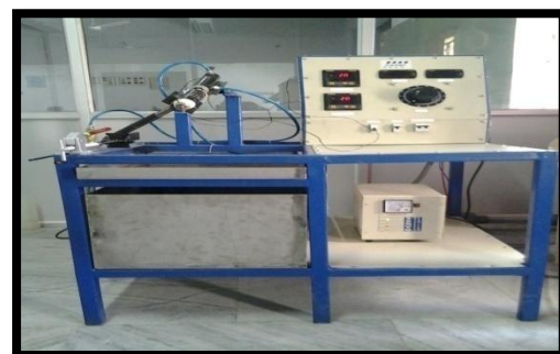
Fig 4.1 Experimental setup of a heat pipe
