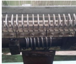
Fig.10. Photographic images of the composite rollers (a) and the energy storage device in the form of a torsion spring (b) of the recommended batan mechanism of the shuttle less loom
