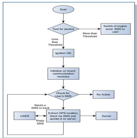
Fig. 2 Flowchart showing the system operation.
