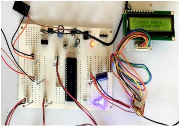
Fig. 5. Alcohol detected, ignition off.
