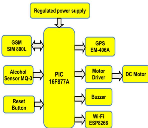
Fig. 3. Hardware Block Diagram of the Proposed System
