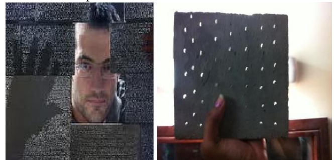
Fig.1. Translucent concrete block.
