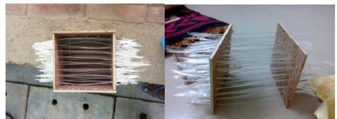
Fig.2 Wooden moulds with optical fibers.
