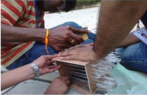
Fig.3. Insertion of optical fiber in concrete mould.
