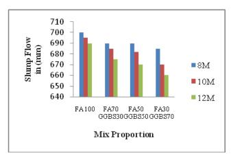
Fig.4. Slump flow test for various molarities.
