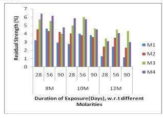
Fig.21: Residual Strength with duration of exposure, wr.t different mix proportion and different Molarities under sulphuric acid attack.
