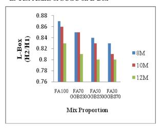
Fig.7. L-Box test for various molarities.
