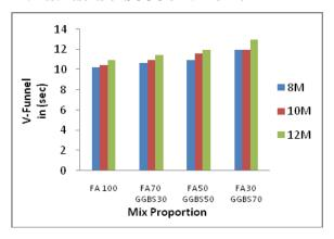
Fig.6. V-Funnel test for various molarities.
