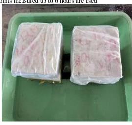
Fig.14.Sorptivity test setup
