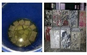
Fig.19.Cubes kept in sulphuric acid medium
