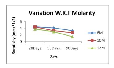
Fig.18. Variation in Sorptivity w.r.t Different Molarity for 70% Replacement of Fly ash with GGBS.
