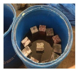
Fig. 13. Absorption test setup
