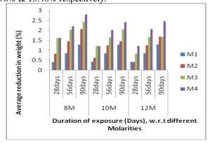
Fig.20. weight loss with duration of exposure.w.r.t different mix proportion and different Molarities under sulphuric acid attack.
