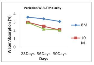
Fig.12. Water Absorption w.r.t Different Molarity for 70% Replacement of Fly ash with GGBS
