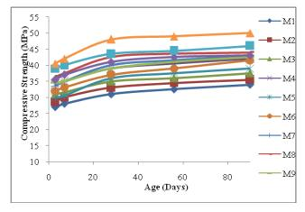
Fig.8. Compressive strength with respect to different binder Components & molarity.
