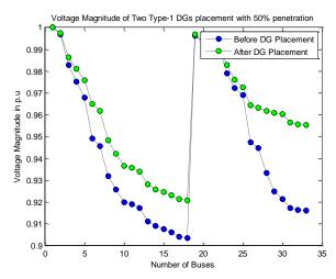
Fig.6. Voltage in p.u of two Type-I DG at 50% penetration
