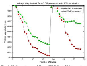
Fig.9. Voltage in p.u of Type-III DG at 50% penetration
