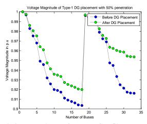
Fig.3. Voltage in p.u of Type-I DG at 50% penetration
