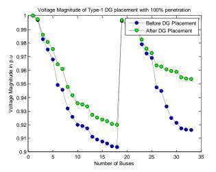
Fig.5. Voltage in p.u of Type-I DG at 100% penetration
