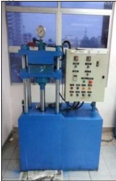
Fig. 1: Hot press machine with FRP curing setup
