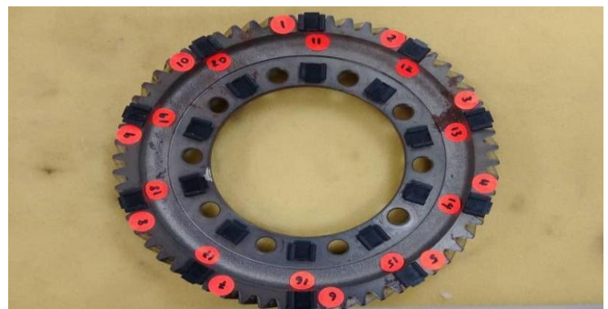
Fig. 2.The healthy condition of the commercially used helical gear
