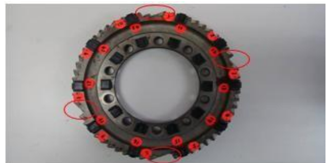
Fig. 3.The unhealthy condition of the commercially used helical gear
