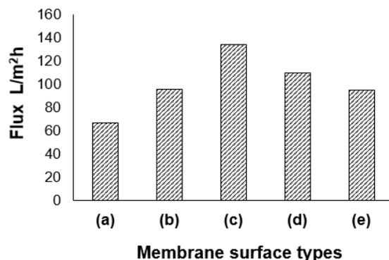
**Fig. 3. Permeated flux for a) Clean PVDF membrane, (b) PDA, (c) PDA/PEI, (d) PDA/PEI/IDA, and (e)PDA/PEI/IDA/ZnO decorated membrane**
