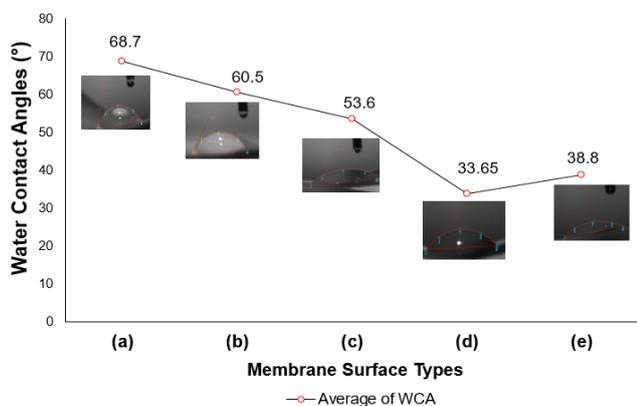
**Fig. 2. WCA for a) Clean PVDF membrane, (b) PDA (c) PDA/PEI, (d) PDA/PEI/IDA, and (e)PDA/PEI/IDA/ZnO decorated membrane**
