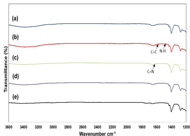
**Fig. 4. FTIR reading for (a) Clean PVDF, (b) PDA, (c) PDA/PEI, (d) PDA/PEI/IDA, and (e) PDA/PEI/IDA/ZnO decorated membrane**
