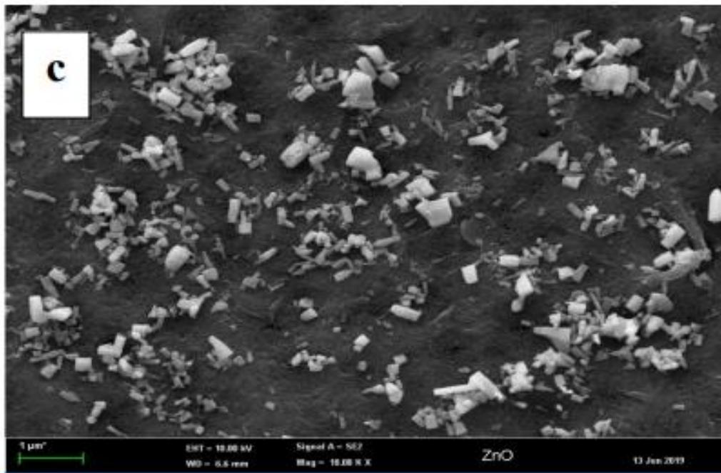
Fig. 5. FESEM Image of (a) Clean PVDF, (b) PDA, and (c) PDA/PEI/IDA/ZnO decorated membrane
