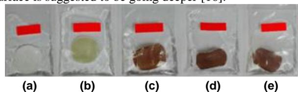
Fig. 1. Colour Observation for (a) Clean PVDF, (b) PDA, (c) PDA/PEI, (d) PDA/PEI/IDA, and (e) PDA/PEI/IDA/ZnO decorated membrane
