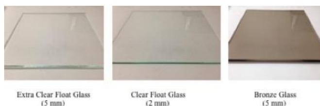
Fig. 2. Condenser plate material
