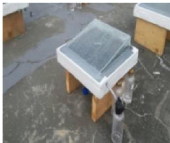
Fig. 4. Single slope solar still
