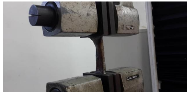
Fig. 3. The skin during Tensile Test.
