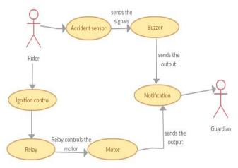
A use case diagram is used to depict the number of users and use cases in a system design including the functionalities of it. The figure attached above shows the use case diagram vehicle security system that we designed to control the accidents and theft of the vehicles.
