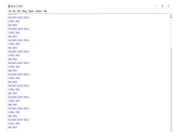
The above screenshot shows the outputs such as 'Accident Alert Minor' and 'Accident Alert Major' which are obtained for different cases when there is minor accident and when there is a major accident and when the motor is in OFF mode.
