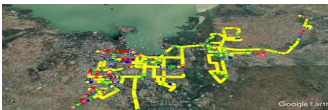
Fig. 2.2: Transmit Power (Ptx) of UE for Cluster network 1 and 2 - Lake Tana – in- and-around together
