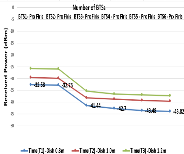
Fig. 3.6 (b) With FT model – the received power for six BTSs
