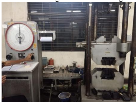
Fig. 4. Tensile strength testing with universal testing machine
