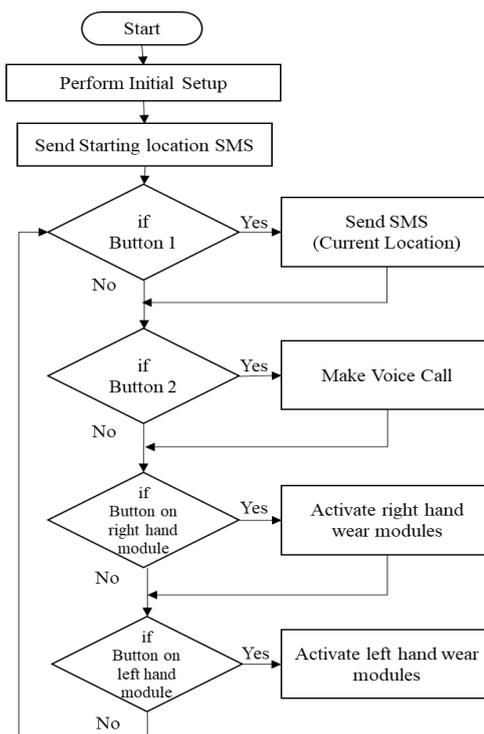
Fig. 8. Flowchart of proposed system software design
