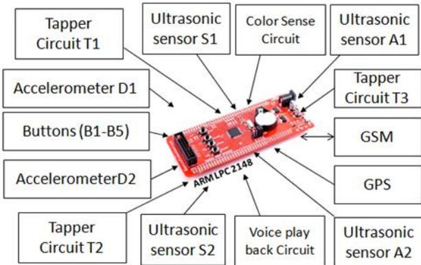
**Fig. 1. Block diagram of the proposed suit and its components used**
