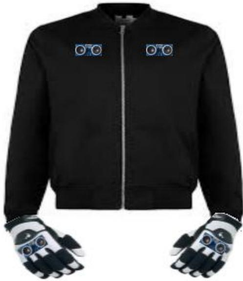
**Fig. 9: Bar tapper Ultrasonic sensors on both shoulders of the jacket.**
