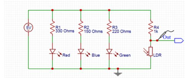
**Fig. 10. Circuit diagram of color sensor Investigation**
