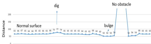
Fig. 8. Ultrasonic sensor output indicating different cases like dig, bulge, normal and abnormal surfaces.
