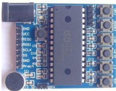
Fig. 3. Voice module with voice feedback
