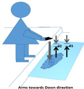
Fig. 6. Sensor detection to detect digs/holes in downward direction ( $d2 > d1$ )
