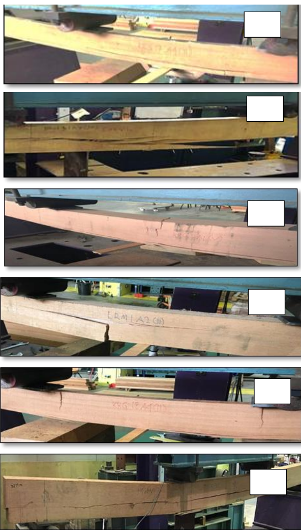
Figure 4: Types of Bending Failure for keruing and light Red meranti.
