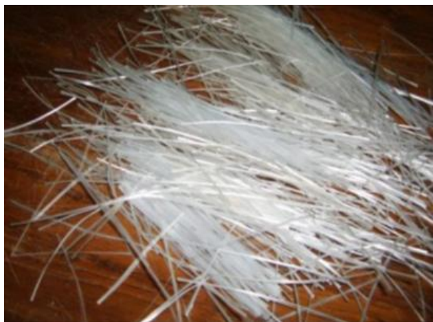
Fig 3. Physical Form of Roving Fiber [1]
