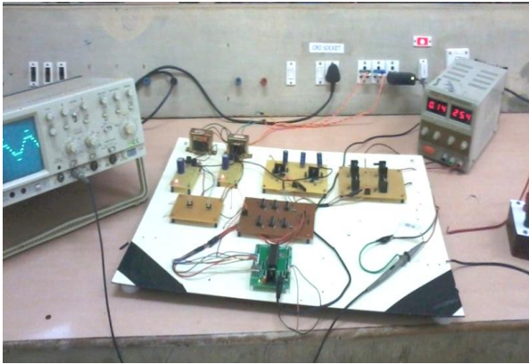
Fig. 10 Inverter Prototype with DC Input from RPS
