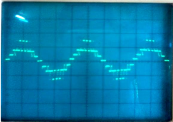
Fig. 11 Output Voltage of Inverter
