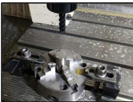
Fig. 1.3 Job Setup with Tool on Machine
