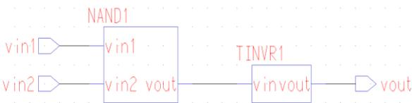
**Fig 2.8: Schematic of ternary AND gate.**
