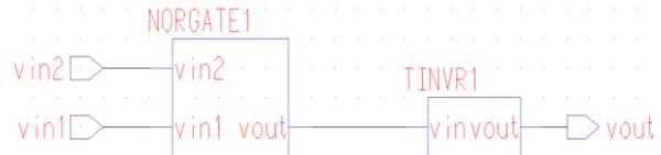
**Fig 2.10: Schematic of ternary OR gate.**
