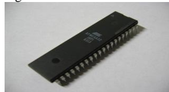
Fig. 2: Microchip Atmega 32A Microcontroller
