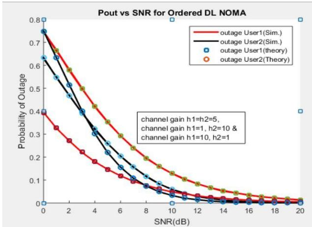
Fig.10. Pout vs SNR for downlink ordered NOMA for various values of channel gains.
