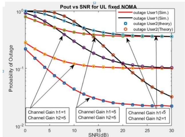
**Fig.9. Pout vs SNR for uplink ordered NOMA for various values of channel gains.**
