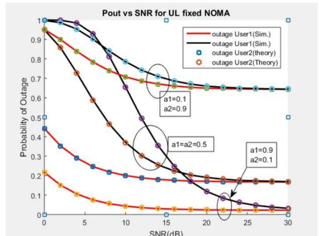
**Fig.8 Pout vs SNR for uplink ordered NOMA for different power factors between 0.1 and 0.9**
