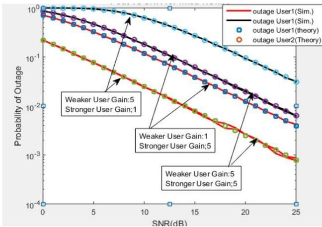
**Fig.6. Pout vs SNR for unordered NOMA for different gain between 1 to 5.**
