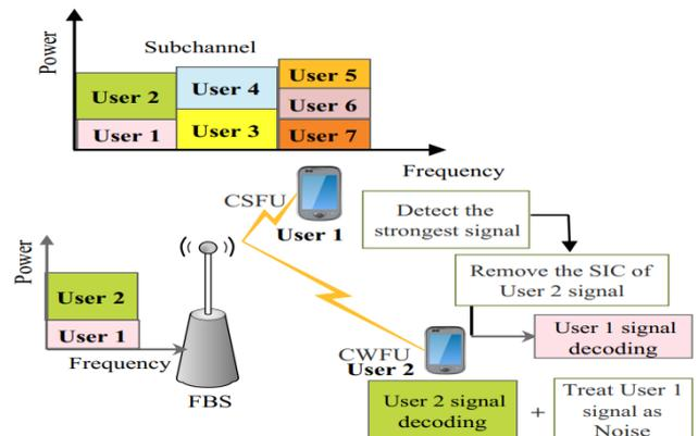
Fig.5. NOMA superposition and Power allocation.
