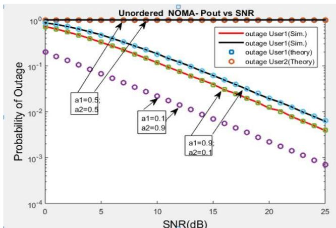
**Fig.7. Pout vs SNR for unordered NOMA for different power factors values.**
