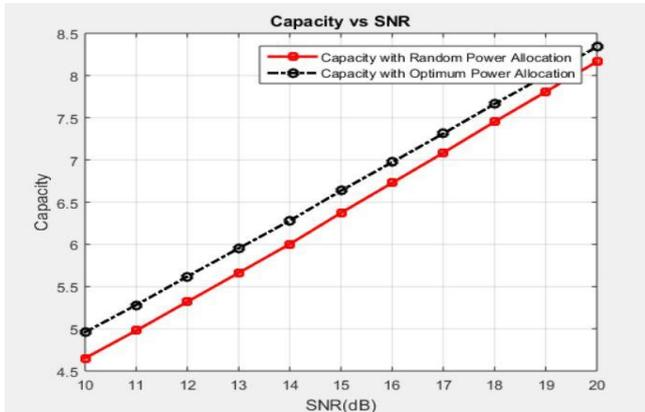
Fig.2. Capacity with random power allocation (SNR) for 0 to 20 dB
