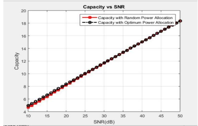
Fig.4. Capacity with random power allocation (SNR) for 10 to 50 dB.
