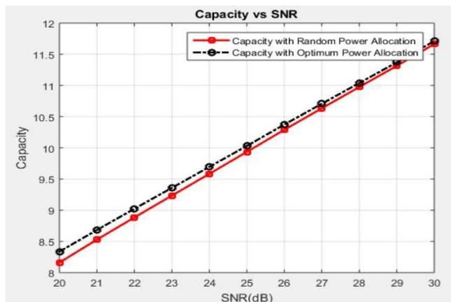
Fig.3. Capacity with random power allocation (SNR) for 20 to 30 dB.
