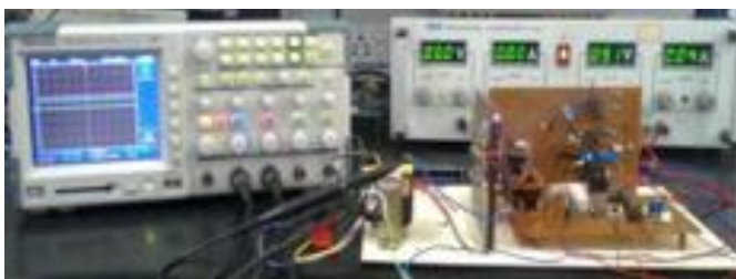
Fig. 7. Three axis Fluxgate Magnetometer with its output
