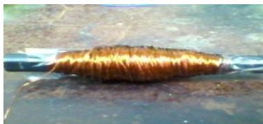
Fig. 5. The coil which is used to create the magnetic field
