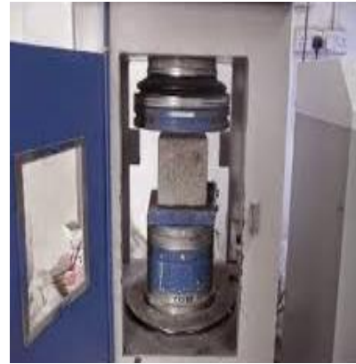
Fig.5 Compressive strength test
