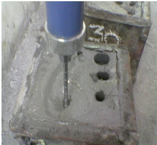
Fig.4 Penetration resistance test
