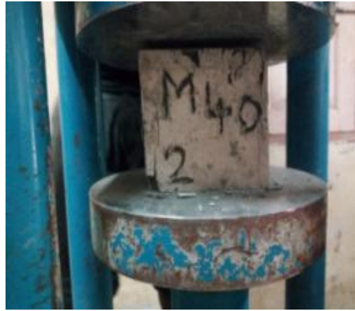
Fig.8. Testing of concrete specimens
