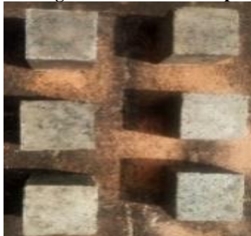
Fig.7. Ambient curing of concrete specimens
