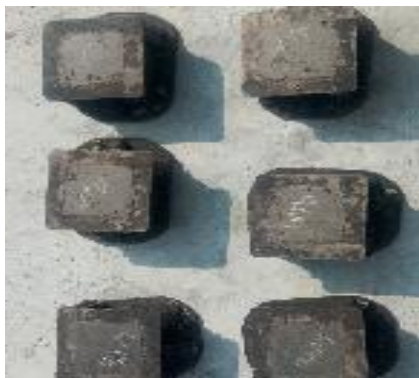
Fig.6. Casting of Concrete Cube Specimens
