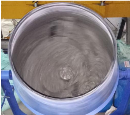
Fig. 10 Mixing of HSCC & HSAAC
