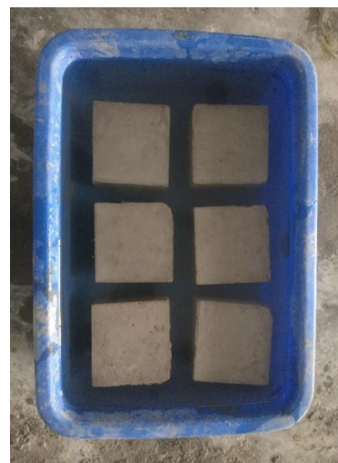
Fig. 14 Sulphate Resistant Test
