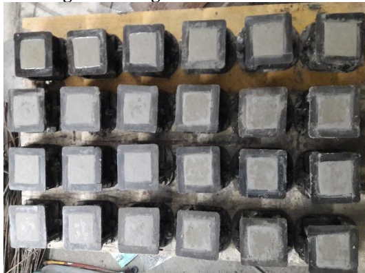
Fig. 11 Cast HSCC and HSAAC Cubes
