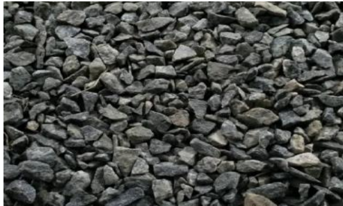
Fig. 7 Crushed Granite Stone Aggregate
