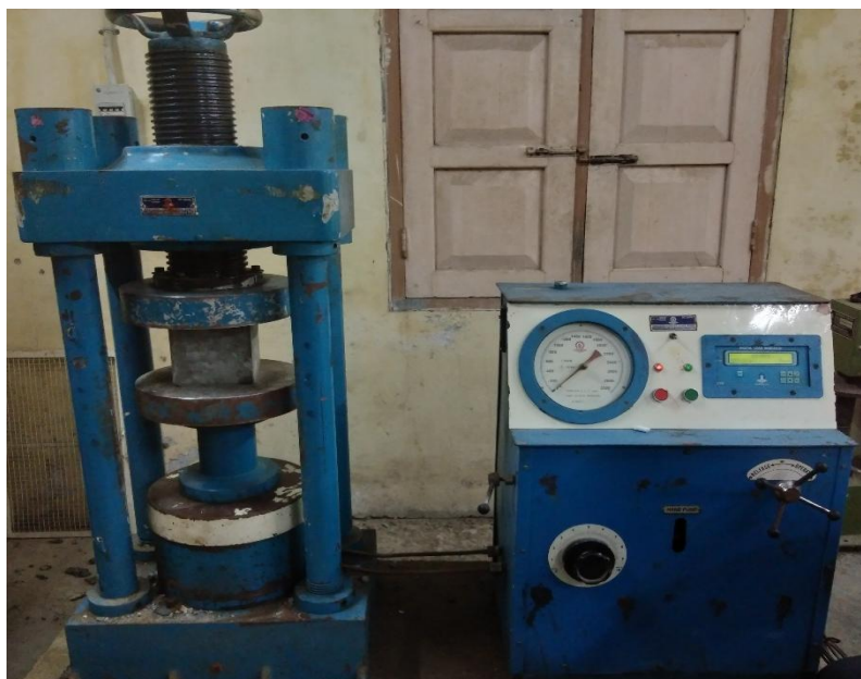
Fig. 12 Compressive Strength Test Setup of HSC cubes
