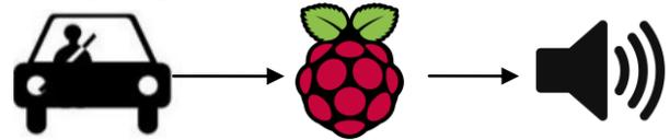
**Fig 2: Pictorial representation of the flow of work, camera will capture video, raspberry pi will process and alarm will turn on if drowsiness is detected**
