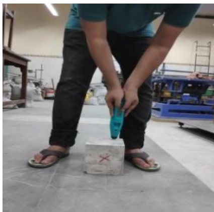
Fig. 6: Schmidt Rebound Hammer Test
