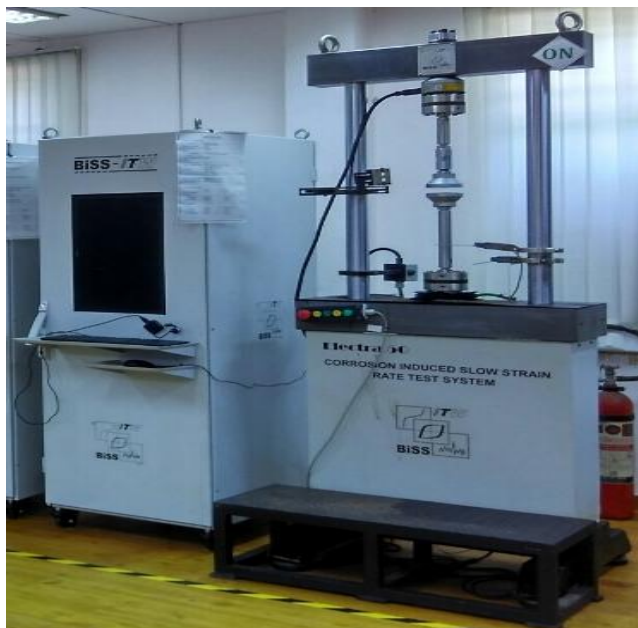
Fig. 2. BiSS Slow Strain Rate Test System
