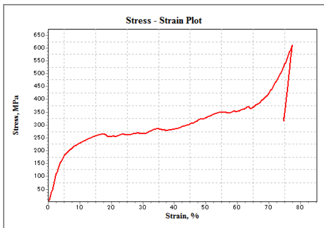
Fig. 5. Stress Strain Curve for 20 v% HGM.
