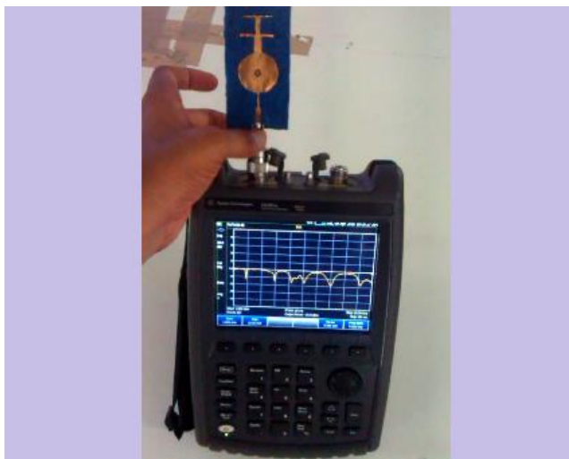
Fig. 6. Validation of Fabricated tri-band antenna with Vector Network Analyzer.
