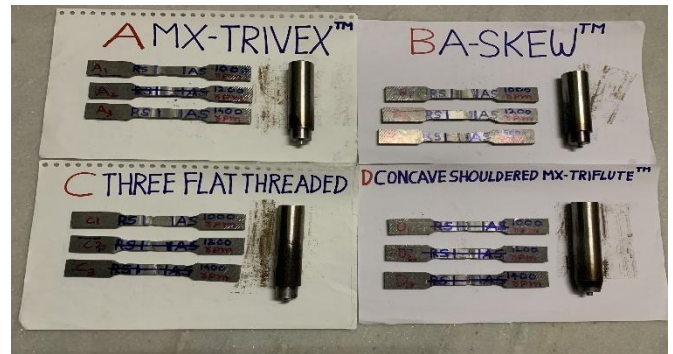
Fig. 15 (a) Tensile test specimens after performing tensile test
