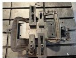
Fig. 2 Clamping of AA6082
