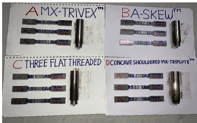
Fig. 12 Tensile test specimens of tool pin profile before performing mechanical test
