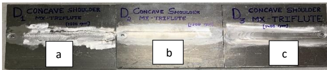
Fig. 9 (a) Concave shouldered MX-TRIFLUTE at 1000 rpm, (b) Concave shouldered MX-TRIFLUTE at 1200 rpm and (c) Concave shouldered MX-TRIFLUTE at 1400 rpm
