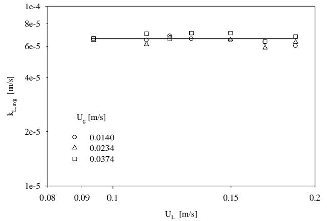
**Fig.5. Effect of gas velocity on  $k_{L,avg}$**
