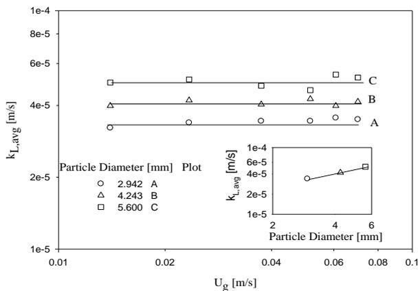
Fig.12 Effect of particle diameter
