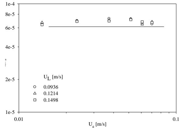
**Fig.6. Effect of liquid velocity on  $k_{L,avg}$**
