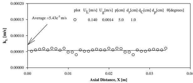
**Fig.4. Longitudinal variation of mass transfer coefficient in three-phase fluidized beds in the presence of inverted cone promoter**
