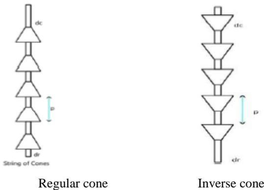
**Fig.2. Configuration of cone promoter { $d_r$  = rod diameter;  $d_c$ = cone diameter;  $p$  = pitch}**
