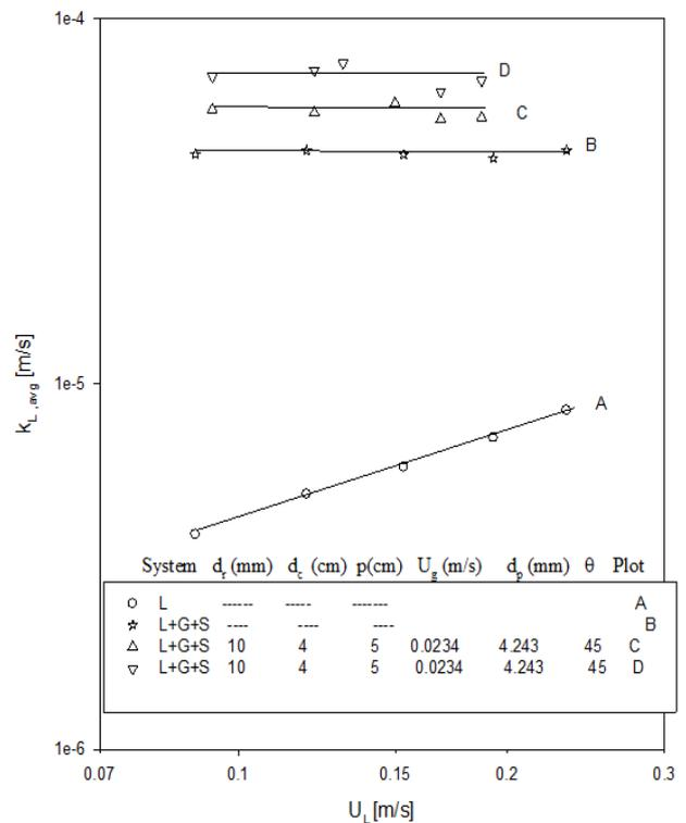
**Fig.3. Augmentation of mass transfer coefficient**
