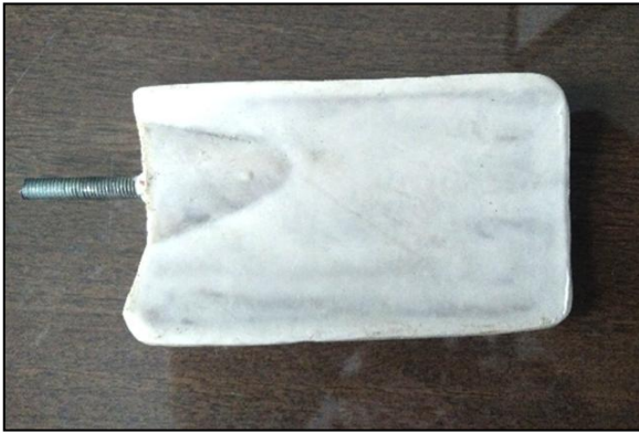
Fig. (8) : Front and Back Side of Composite Fan Blade
