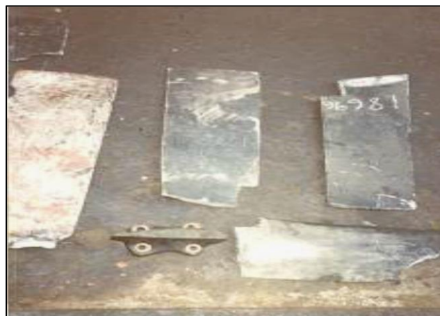
Fig. (1) : Blade Failure Due to Improper Heat Treatment
