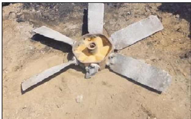
Fig. (2) : Blade Damage Due to Pressure Variations
