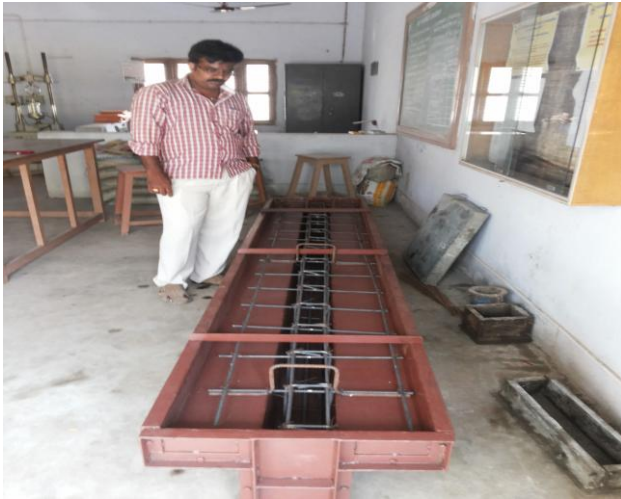
Fig 1. Tee beam mould with reinforcement bars
