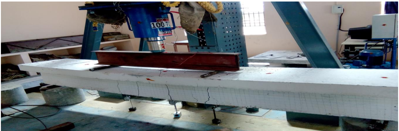
Fig 4. Flexural Testing on Tee beam Specimen
