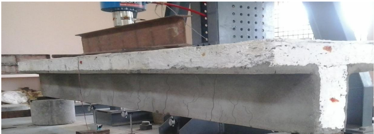
Fig 7. Flexural Testing on Strengthened Tee Beams
