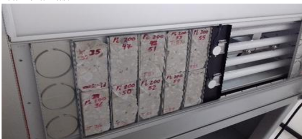
Figure 2 Placing specimens in the EEA chamber. Source: Photograph of the authors
