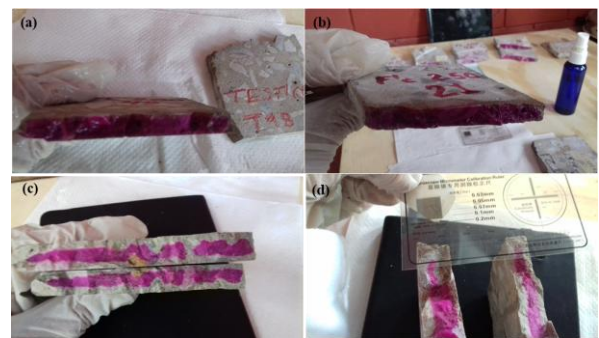
Figure 4 Test to determine the carbonation front with phenolphthalein. (a) Tablet f'c = 200 \text{ kg / cm}^2 of Control. (b) Tablet f'c = 250 \text{ kg / cm}^2 of Control. (c) Tablet f'c = 200 \text{ kg / cm}^2 with 180 hours in EAA. (d) Tablet f'c = 250 \text{ kg / cm}^2 with 180 hours in EAA. Source: Photograph of the authors.
