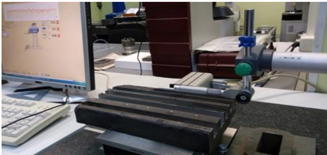
Fig. 9. Obtaining profilogram of the surface of profile (Hommelwerke profiler-profilometr).
