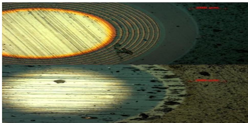
Fig. 3. Microsections of samples with coatings: a) TiAlN, b) nACRo3®
