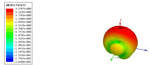
Figure 1.6. Directivity plot of the 2 element antenna array with element spacing \lambda
