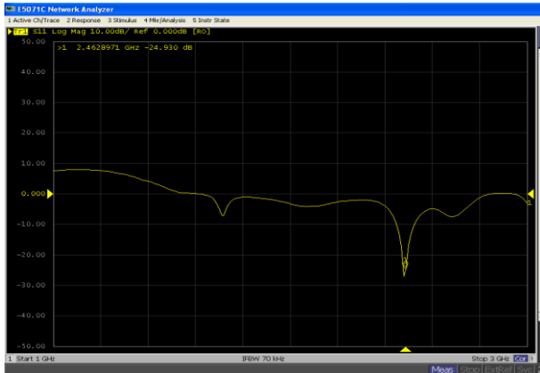
Figure 1.14. Reflection coefficient curve of the fabricated 2 element antenna array with element spacing \lambda
