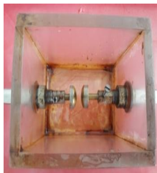
Fig 1. Front view of breakdown voltage measurement setup. Fig 2. Test cell of the breakdown voltage setup.
