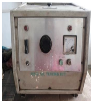
Fig 1. Front view of breakdown voltage measurement setup. Fig 2. Test cell of the breakdown voltage setup.
