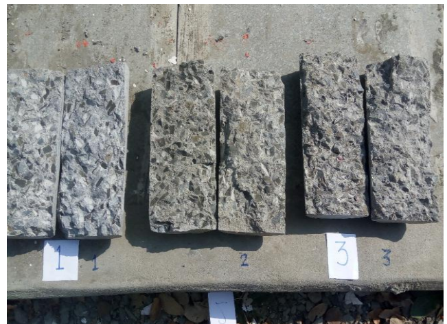
Fig. 10 Specimen failure pattern for splitting tensile test (after testing)
