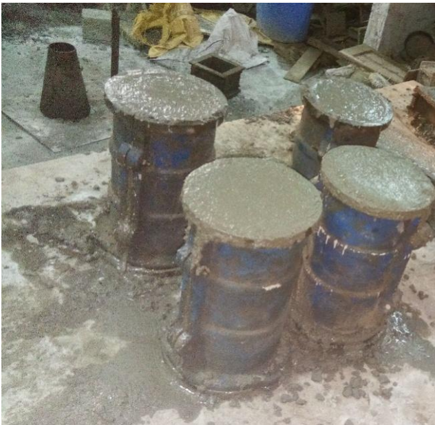
Fig. 9 cylinder specimen mould for splitting tensile test
