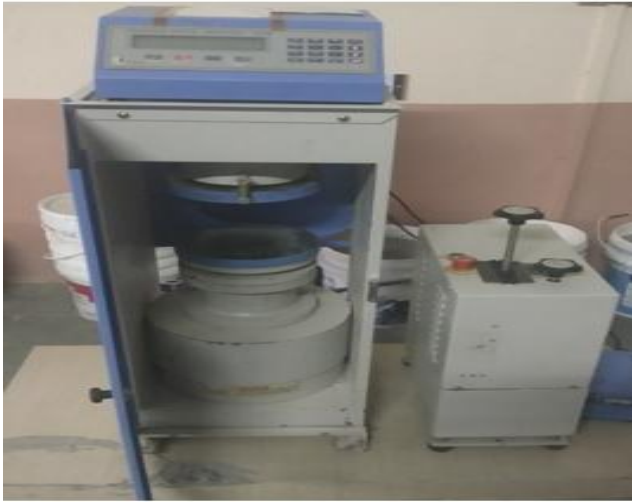
Fig. 1. The experimental set up of CTM for compression tests
