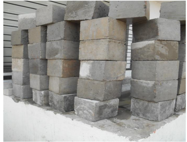
Fig. 2. Concrete Specimen cubes (150mm x 150 mm x 150 mm) before testing
