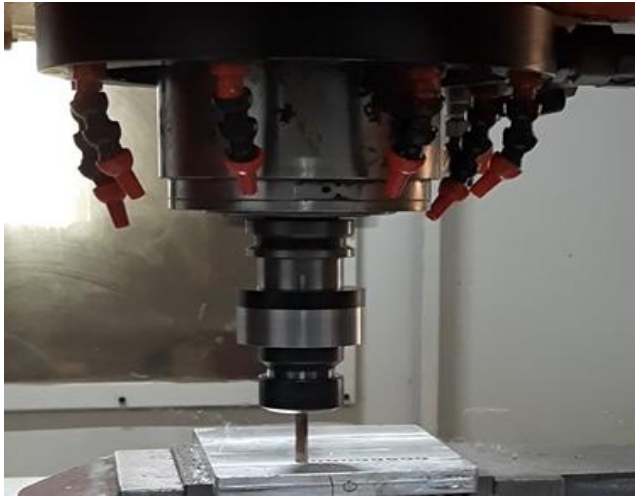
Figure 2: Drilling of Aluminum metal matrix composites
