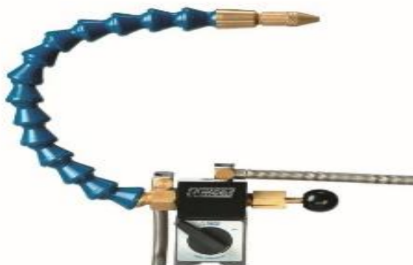
Figure 3 .Minicool MQL Setup
