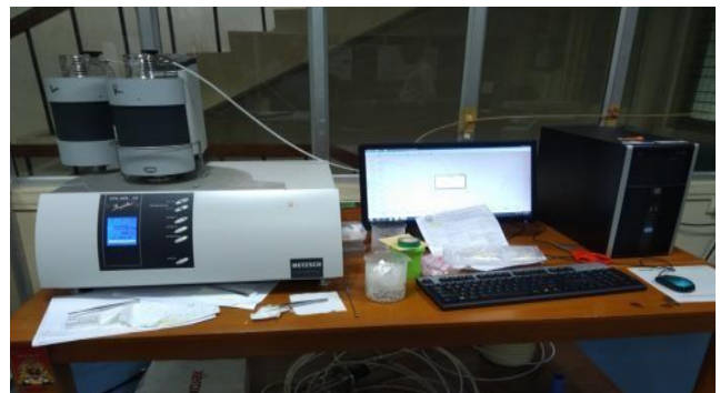
Fig:1. TG-DSC instrument Make NETZSCH STA 449F3
