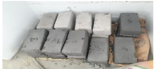
Figure 3 De moulding of BMSS Bricks
