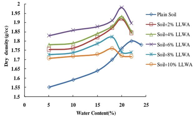
**Fig. 3. Variation of dry density with moisture content for different LLWA contents**
