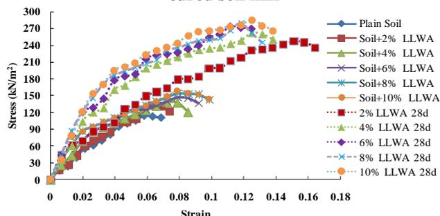
Fig. 5. Stress vs strain relation for uncured and 28 day cured soil mix
