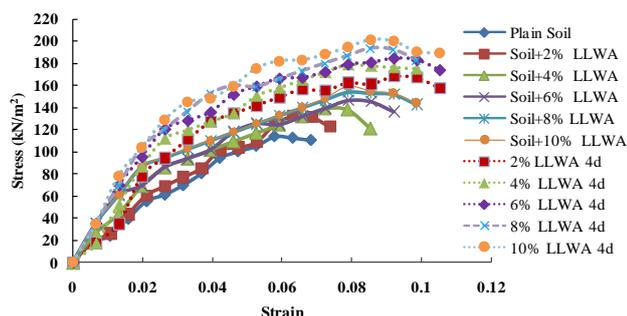
Fig. 4. Stress vs strain relation for uncured and 4 day cured soil mix
