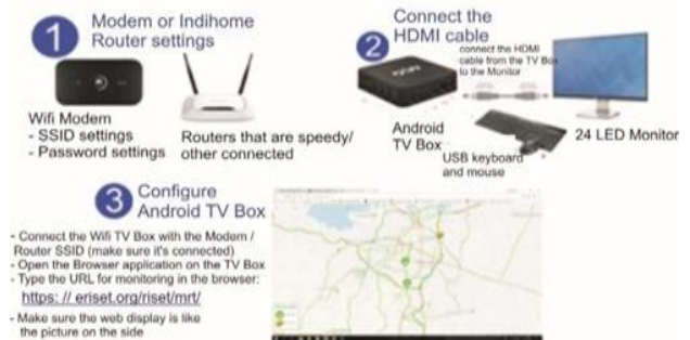
Figure 8. Monitoring System Configuration to display coordinate data on the Passenger Information System
