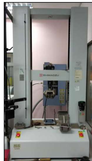
Figure 3: Shimadzu Testing Machine with 50 kN Capacity
